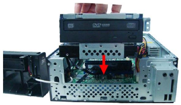
2. Secure the HDD-ODD bracket to the chassis using two screws.
